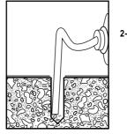
2.Clean each anchor hole thoroughly using a vacuum cleaner with a narrow nozzle attachment to reach into the hole and remove all debris.
