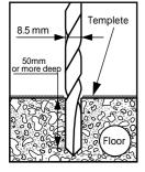
1.Drill the anchor holes of a speci c diameter and depth.
