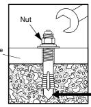
4.Adjust the fastening strength of the nut using a wrench etc.
