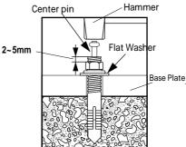
3.Insert the anchor bolt, tapping it lightly with a hammer to seat it. Position the material, and then drive the center pin into the anchor unit it is snug.
