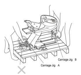
Do not make scratch or damage he oor while moving the unit. Please use the carriage jig to move it.
